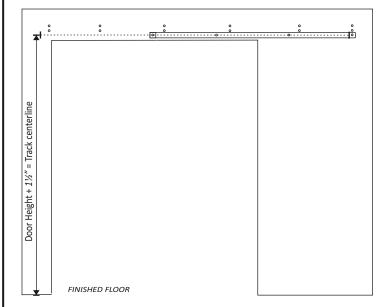
Use the front track to determine the spacing for the bypass bracket pilot holes.
