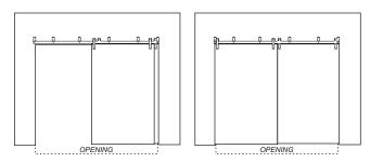
Where doors slide freely, in either direction and stack within the opening to leave only one side of the opening clear.
