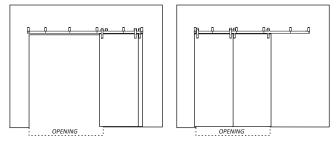
Where doors stack collectively on either or both sides of the opening to leave the opening clear and free from obstruction.
