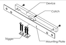
NOTE: Instructions apply to all standard 11 inch and 17 inch Soft Stop systems. Custom hole patterns over 11 inches can be made available upon request
