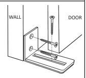
Tip: Optionally, the remaining wood screw may be inserted into the floor through the middle of the bottom slot in the L bracket.
