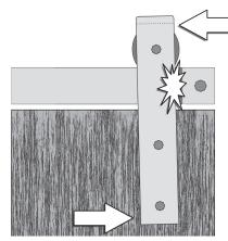
The hangers are not bending. Instead, the hanger mounting bolts are moving just a bit, and pushing against the mounting holes in the door.
